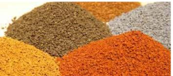
Natural Stone is used for all quality MRT. However, different types of rock have different properties. They should not only be hard and strong, but also UV stable to ensure colours do not change under Ultra-violet exposure. It is also important that the stone has a low iron-content to prevent patches of rust appearing on the tiles and discolouring the roof.
