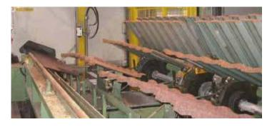
The first stone coated tiles made in New Zealand over 60 years ago used bitumen to bond the stone coatings to the base metal. After long UV exposure, the bitumen began to crack and 'chip-loss' started to occur. Today, the world's biggest companies have developed their own acrylic based coating technology. The Intellectual
